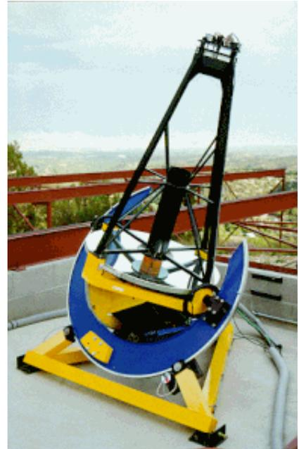
Tennessee State/Smithsonian 0.80m Automatic Photoelectric Telescope
